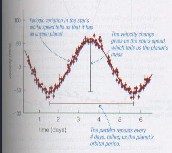
a A periodic Doppler shift in the spectrum of the star 51 Pegasi shows the presence of a large planet with an orbital period of about 4 days. Dots are actual data points; bars through dots represent measurement uncertainty.
