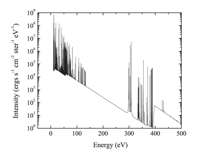
FIG. 13. Model spectrum from a steady-state simulation with  $T_e=30$  eV and  $n_i=5 \times 10^{14}$  cm<sup>-3</sup>. Impurity concentrations of 1% carbon, 0.002% oxygen, and 0.003% nitrogen were included. The plasma emits primarily at E < 150 eV, but SXR will also measure substantial emission from the C v and C vI resonance lines between 300 and 400 eV. Note that the Zr channel has the lowest responsivity at these energies, which is counter to what is seen below 100 eV.
