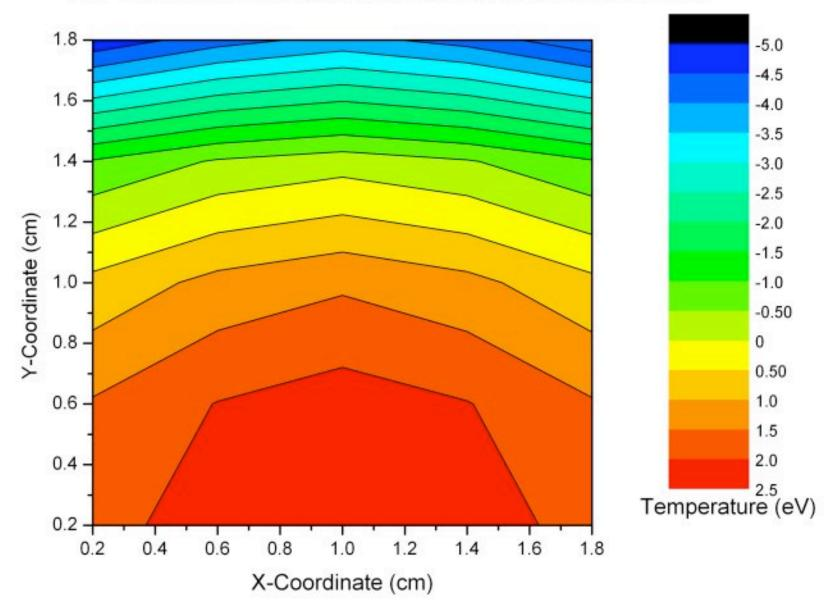
Gas Cell Radiation Temperature Departure from Mean at 100 ns
