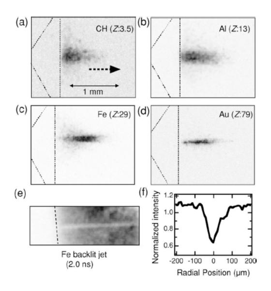
FIG. 2. Snapshots of two-dimensional side-on self-emission images from the XFC for (a) CH, (b) A1, (c) Fe, and (d) Au targets at 1.3 ns after the laser irradiation. (e) Backlit Fe jet image from the XFC at 2.0 ns, and (f) radial lineout plot at 1 mm from the center of the cone target.
