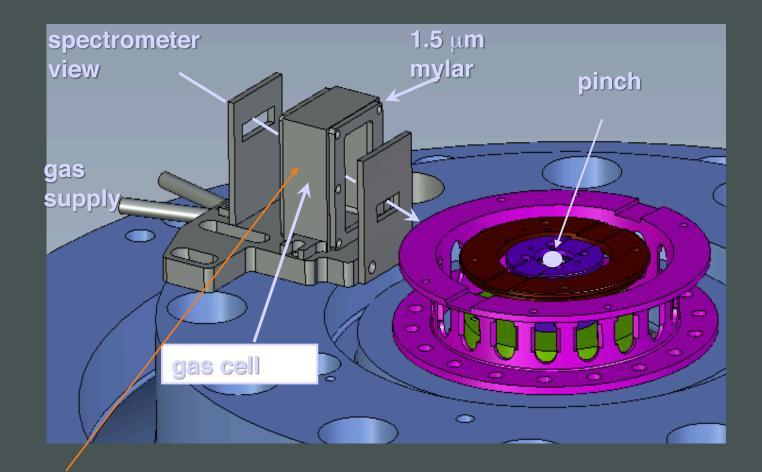
Side view with second spectrometer – measure recombination spectrum
